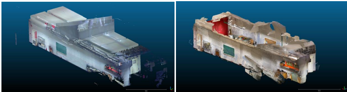
Figure 6: Unedited point clouds of A-17. TLS point cloud (left) and Modelar's iPhone point cloud (right)
