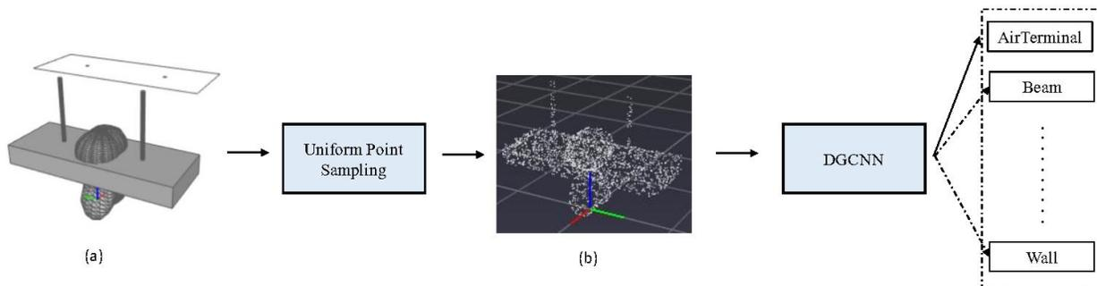
Figure 1: Pipeline of 3D IFC object classification with DGCNN; a) IFC object b) generated points using uniform sampling.
