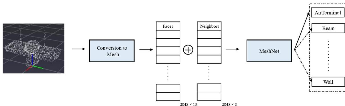
Figure 2: Pipeline of the 3D IFC object classification using MeshNet.
