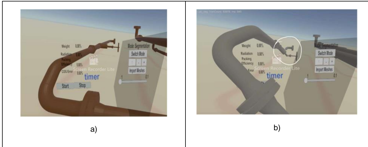
Figure 4: Screenshots of the decompose mode. (a) The semi-transparent square indicating the cutting direction. (b) Unwanted cuts being generated using Mesh Slicer
