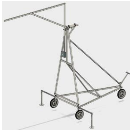
Figure 1: Model of original TIA design used to inspect Grand Falls tunnel (Bradley 2018)
