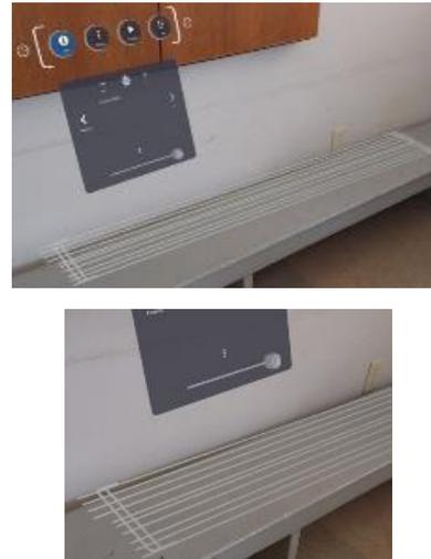
Figure 14: A representation of reinforcing objects in the TCH application when using the sequence tool. All objects shown in one color regardless of their classified color in the design model.
