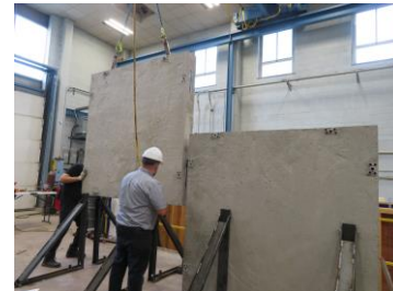
(b) Placement of second wall panel
