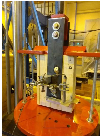
Figure 2 Type 3 setup with LVDTs.
