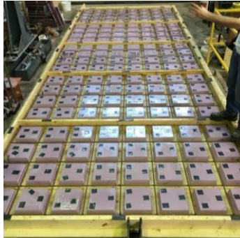
Figure 3: Shaker Table and Forms Prior to Concrete Pour
