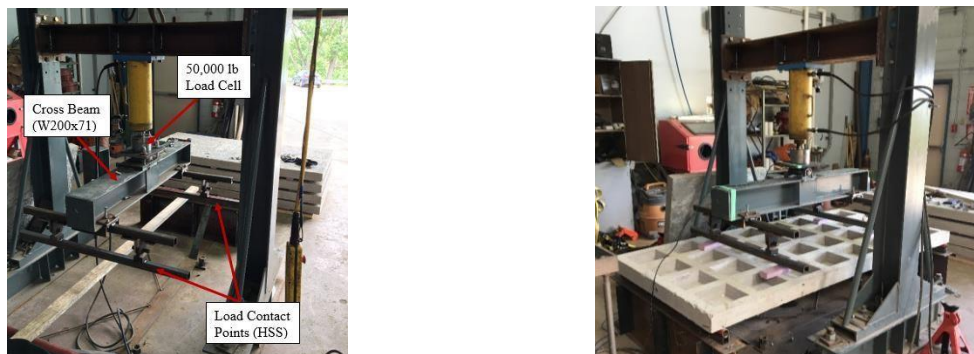
Figure 4: Testing Apparatus Used for Panels Under Pure Flexure
