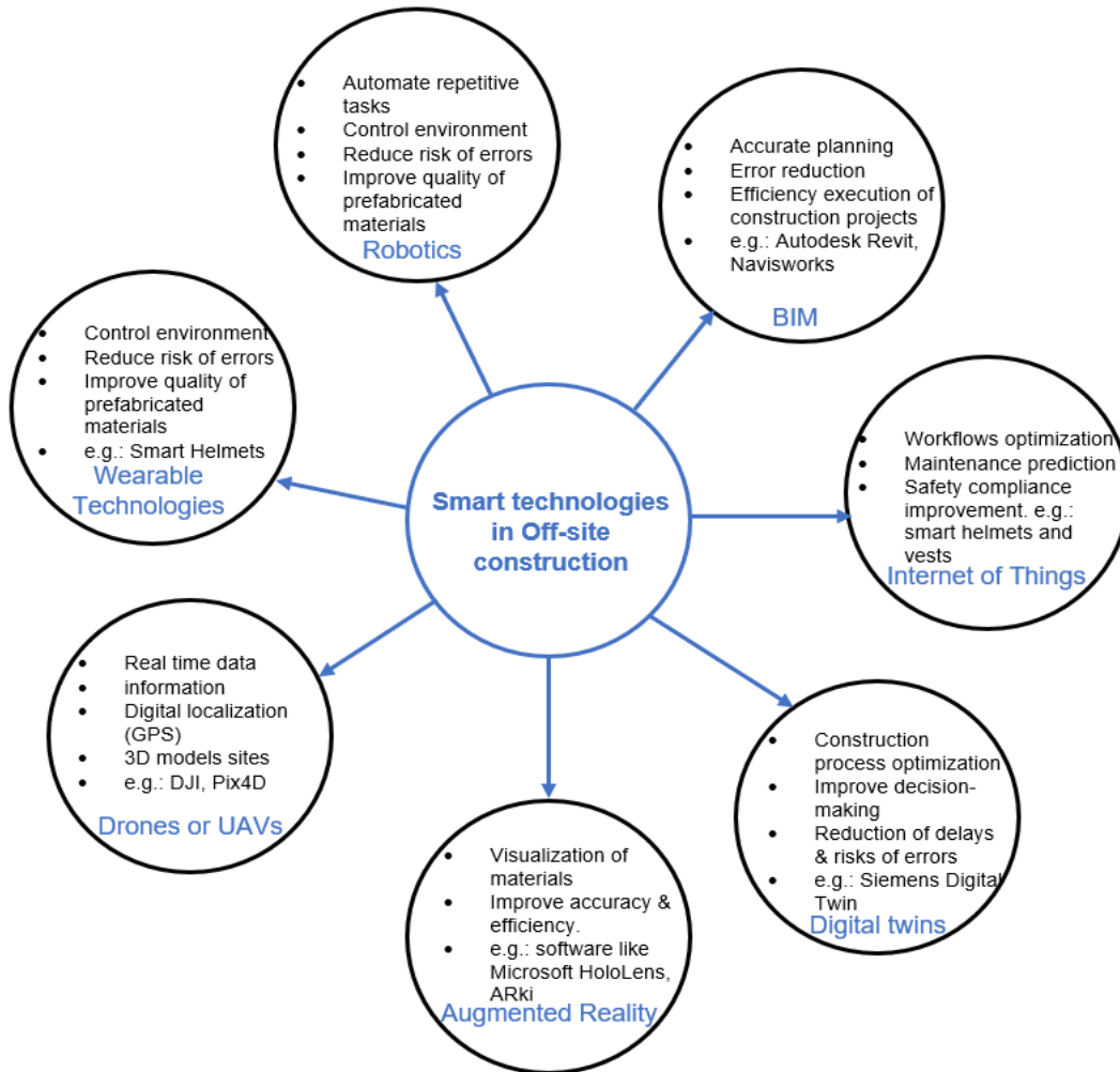
Figure 3: Smart technology functionality in offsite construction
