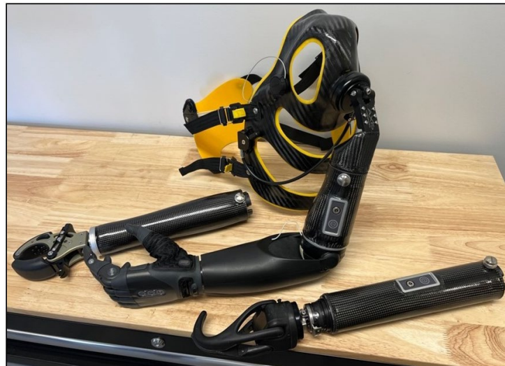
Figure 3: Final Prosthesis with three interchangeable arm segments
