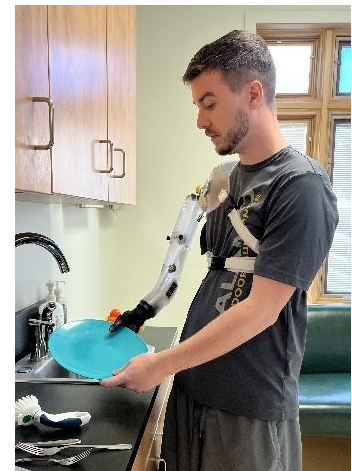
Figure 3: Novel shoulder disarticulation prosthesis in its extended position to work at a countertop height while standing
