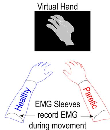
Figure 1: Experimental Setup. Participants were instructed to mimic the preprogrammed movements of the virtual arm with their healthy arm or paretic arm. EMG activity was recorded using a symmetric bilateral pair of custom 32-electrode EMG sleeves.
