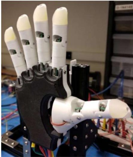
Figure 1. The BEAR PAW: a pediatric multiarticulate prosthetic hand with six degrees of freedom and programmable grasp configurations.
