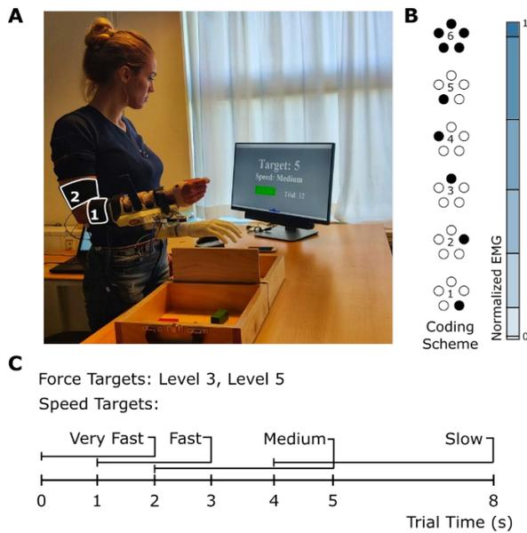
**Figure 1: Experimental setup.** (A) Experimental setup shows a participant using (1) 2-dry EMG electrodes and (2) 5 vibrotactors to perform a modified box-and-blocks task over 3 days. (B) Spatial coding scheme to convey EMG biofeedback through vibrotactors. (C) Force and speed targets (restrictions) for the task, used to derive a speed-accuracy trade-off.
