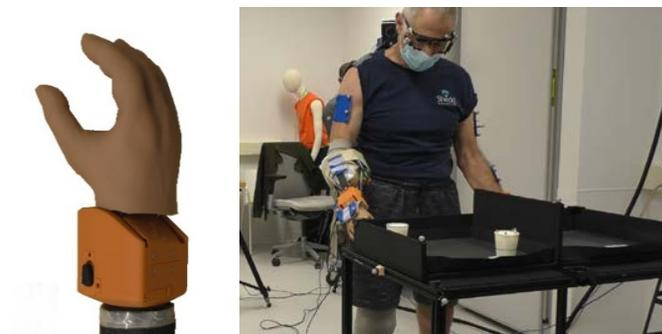
Figure 1: a) Device used for the study. b) Participant wearing the device, in “home” position, ready to begin the Cup Transfer Task.
