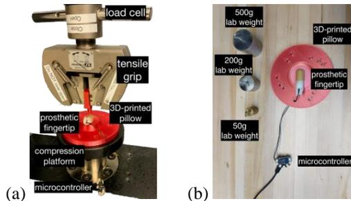
Figure 2: (a) Data collection setup using a universal test machine and a custom-made pillow for the fingertip sensor. (b) Experimental setup to collect real-time prediction results from the fingertip.
