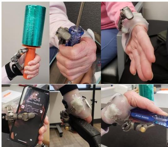
Figure 4: Patient demonstrating the ability to achieve a variety of oppositional grasps to hold various objects as well as a flat hand posture to maximize use of the intact digits.
