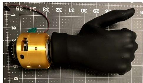
**Figure 1:** Prototype VAPI with iLimb Hand
