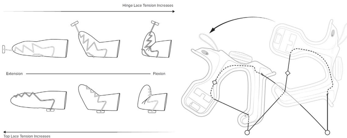
Figure 5: Diagram showing the changes in tension of the dynamic lace systems throughout (left), and of the four hinge crossings of the hinge lace loop, showing how the lace moves through the elbow counter (right).
