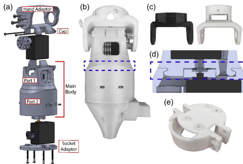
**Figure 1:** **A)** Exploded view of the Utah Wrist. **B)** A photo of the assembled wrist with the attachments to connect to a bypass socket. **C)** The wrist can adapt to a variety of different terminal devices by printing a new interface part such as the two shown here. **D)** Expanded view of the rotary joint mechanism, as highlighted in part B. **E)** The wrist can connect to different kinds of sockets by printing out a new interface such as the part shown here.
