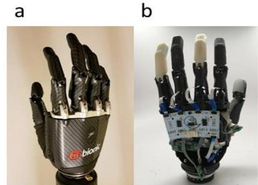
**Figure 5:** (a) Commercially available Bebionic v2 hand (b) Modified Bebionic hand used for finger actuation experiments. Custom electronics were installed in order to control individual motors within the prosthesis. The Bebionic has motor encoders that can measure finger position and be used in closed-loop control.
