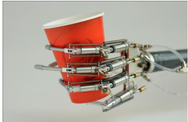
*Figure 2 - The prototype of the Delft Cylinder Hand. It has four adaptive fingers actuated with two hydraulic cylinders in each finger, except for the little finger which has only one hydraulic actuator. The springs return the fingers to the open position at rest, and partly compensate for the counteracting forces of the cosmetic glove (not shown in the picture) as well. The cylinders in the hand receive the pressurized hydraulic fluid from a master cylinder incorporated in a shoulder harness.*
