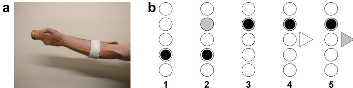
Figure 1: (a) Example bypass socket. (b) Visual prompts used in vertical arm position experimental protocol. 1: Participant views five vertical positions with current position highlighted. 2: Target position is presented. 3: Participant moves arm to target position. 4: Prompt indicates to activate the flexor (left arrow) or extensor (right arrow). 5: Feedback may be presented if muscle activity reaches threshold value.
