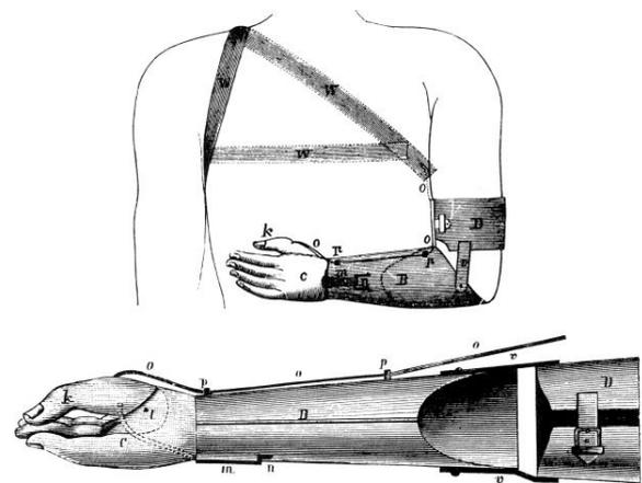
*Figure 1 - Prosthetic forearm designed by Count De Beaufort in 1860. The hand is controlled by a cable, indicated by O, which is attached to a shoulder harness.*
