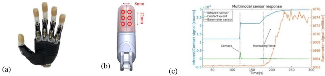
Figure 1: (a) The Point Touch integrated into the Bebionic hand. (b) High-level sensor architecture (c) Sensor response when a small piece of cotton is dropped onto the sensor and pressed.
