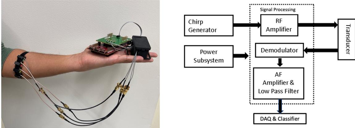
Figure 2. *Left*: The prototype of our 4-channel wearable ultrasound system. *Right*: System diagram of the hardware components.
