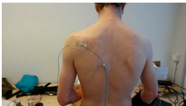
Figure 3 – The skin anchors placed on the body of a test subject. The cables are connected to the experimental set-up used to verify the idea behind the haptic interface.
