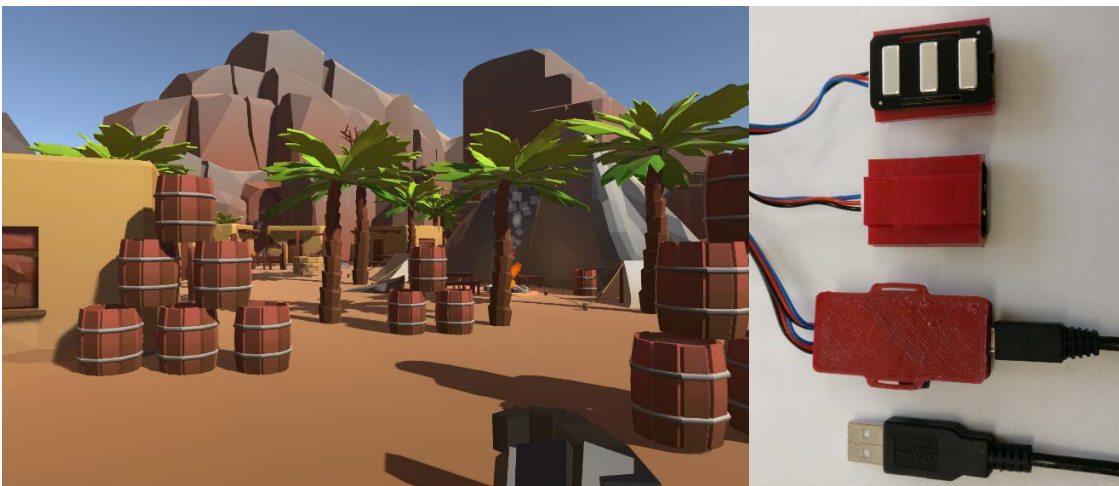
Figure 2: Images from iteration two. Left: game scene based on purchased assets. Right: microprocessor game controller, signal processing and IMU unit and two dry EMG electrodes.
