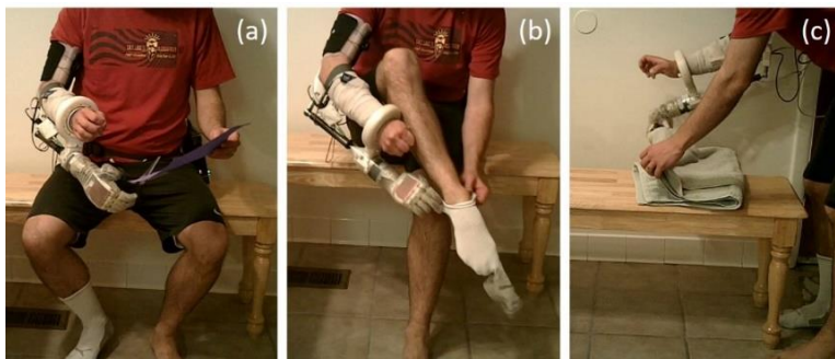
Figure 2 - Two-handed activities-of-daily living in the home using a bypass socket and the portable system: (a) using scissors, (b) donning a sock and (c) folding a towel.
