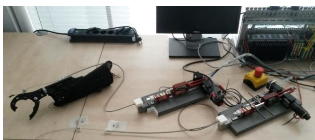
Figure 4 – The experimental set-up. On the left the prosthetic simulator; in the middle and right part of the figure the master-slave unit is shown. Also visible are the cables and on the foreground, the skin anchors.
