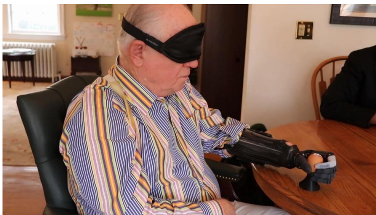
Fig. 4 Subject S2 successfully grasping the eggshell when receiving touch feedback while blindfolded.
