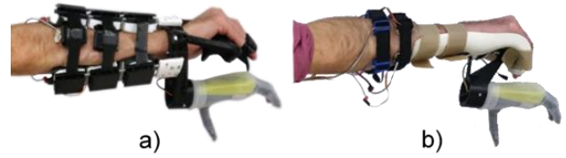
Figure 3: A participant wearing a) the Modular-Adaptable Prosthetic Platform as a simulated prosthesis and b) the orthotic splint.
