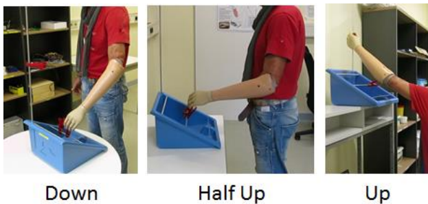
Figure 3: Evaluation in the clothespin relocation test, executed in three different arm positions
