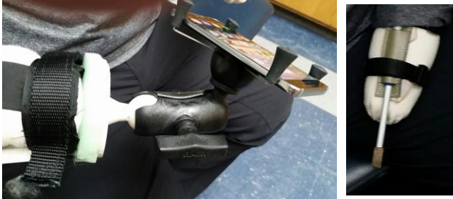
Figure 8: Smart phone configuration with commercially available RAM Mount attached to the right prosthesis and a stylus attached to the left limb
