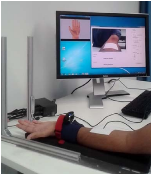
Figure 1: The experiment setup, where a subject is following the stimuli on the monitor with a sticker stuck on to the left forearm and a camera attached to the arm to capture its deformations
