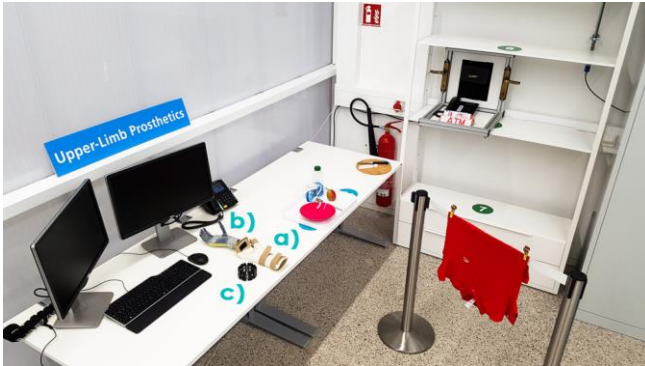
Figure 1: overview of the laboratory setup including a) the i-LIMB on an b) orthotic splint, c) the Myo bracelet and daily-living objects that were manipulated during the experiment.
