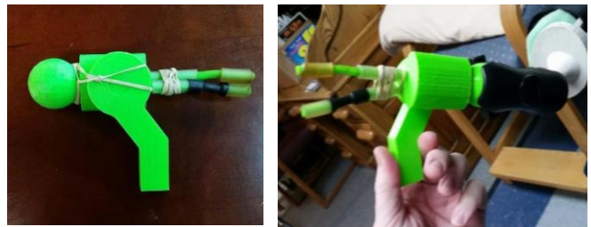
Figure 6: Printed prehensile device with rubber bands providing closing force
