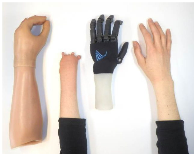
Figure 9: Restorative treatment, left: previous conventional prosthesis; right: example of treatment from Pohlig GmbH with VINCENTpartialhand components.
