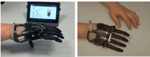
Fig. 6: Test version of a myoelectric partial hand prosthesis with integrated controller and battery
