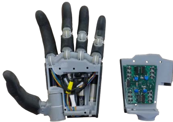
Figure 2. Hand with cover removed, showing embedded system and motor units.
