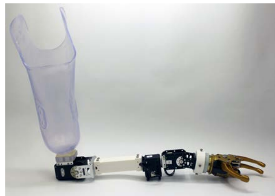
Figure 3 – The Bento Arm integrated with a test socket
