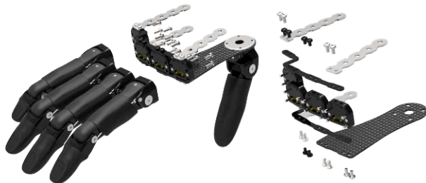
Figure 3: Modular, anatomically size partial hand system: frame with slight abduction for four finger and an active thumb, left hand.
