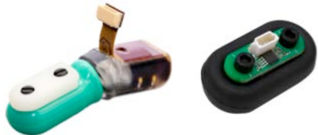
Figure 1: Left - a BioTac® tactile sensor; Right - a low-cost NumaTac® prototype tactile sensor.
