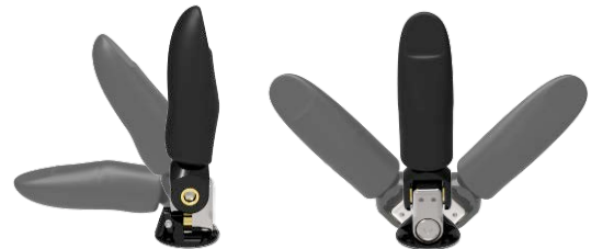
Figure 5: Two axes scope of movement of the passive thumb, the proximal joint with motion resistance (ri.) and the distal joint with ratchet-type (le.).
