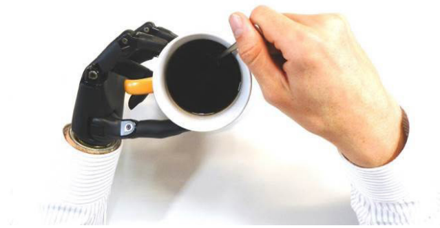
Figure 5: Thanks to a force feedback system, objects can be gripped precisely even without direct eye contact: hand in Vincent-handlegrip.
