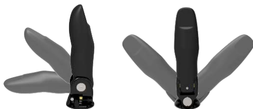
Figure 7: Two axes scope of movement of the active thumb, the manual proximal joint (ri.) and the motor driven distal joint (le.).
