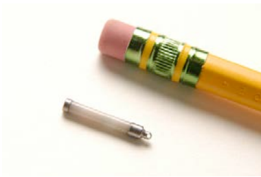
Figure 1: IMES®, implantable myoelectric sensor
