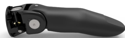
Figure 6: Active thumb with powered distal joint and stepless passive proximal joint, soft thumb-tip.
