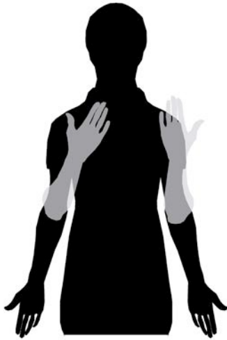
Figure 1. Human elbows (left) have a natural carrying angle, that causes the hand to be more lateral than the elbow when fully extended. This carrying angle has an important effect during elbow flexion, causing the hand to move closer to the midline. In contrast, conventional prosthetic elbows (shown on the right side of the image) flex the forearm straight up, no closer to the midline, and thus require humeral rotation to reach the midline.
