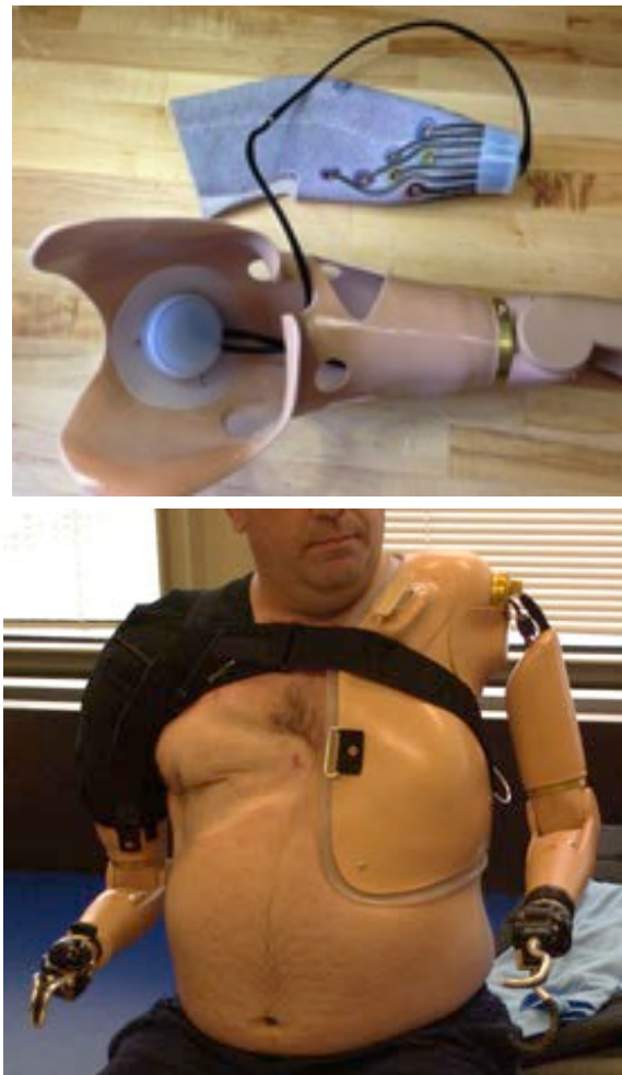
Figure 2: Top: Experimental APR system embedded in socket. Bottom: Final laminated system with commercial Complete Control APR controller
