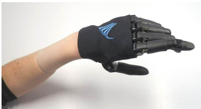
Figure 1: Example of partial hand system with four active long fingers and an active thumb with a biomechanically optimized shaft structure.
