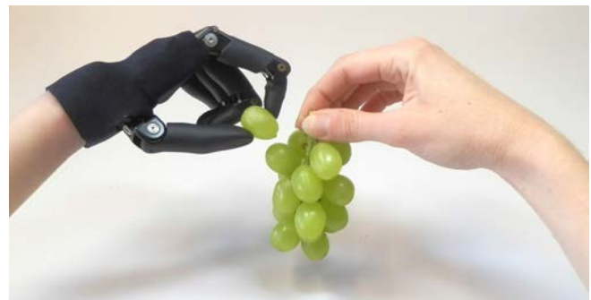
Figure 12: Fully integrated partial hand with 4 active driven single fingers and an active driven thumb allows a fine manipulation.
