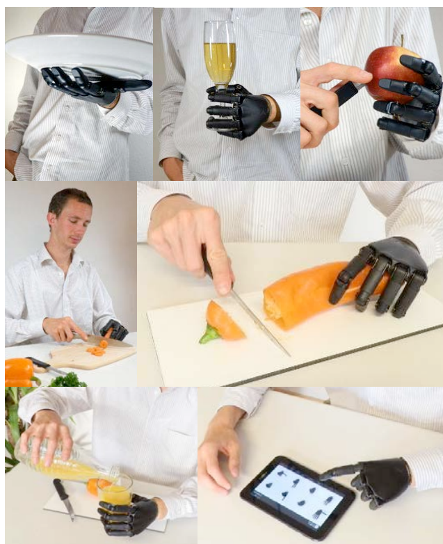
Figure 7: Training with the hand prosthesis, using the Vincent-app : the interactive training program communicates with the prosthesis control unit: training of tablet-, Vincent-cupholder -, zylinder- and indexgrip at work.
