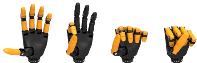
Figure 2: Lateral movement of the VINCENTevolution2 and opposable thumb to the ring finger.
