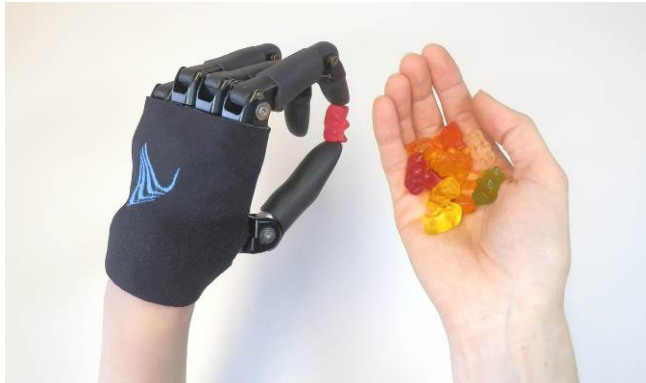
Figure 14: The precision grip can be used to grab and hold small objects.
