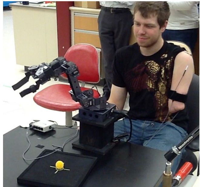
Figure 1: Amputee participant performing simple tasks with the robot arm using myoelectric control signals
