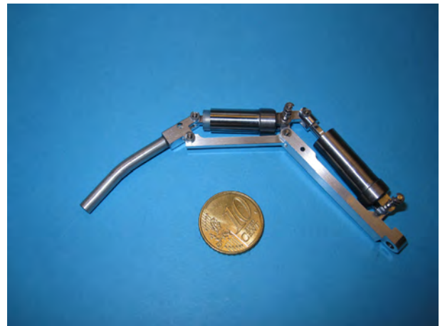
Figure 2: One of the three 2DoF hydraulic fingers. The finger is activated by the small metal cylinders.
