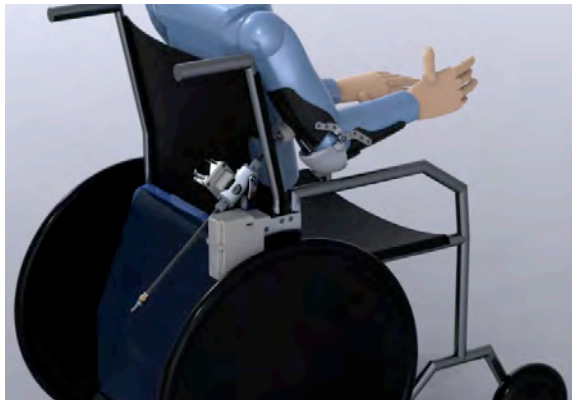
Figure 1: OrthoJacket system, mounted on a wheelchair
