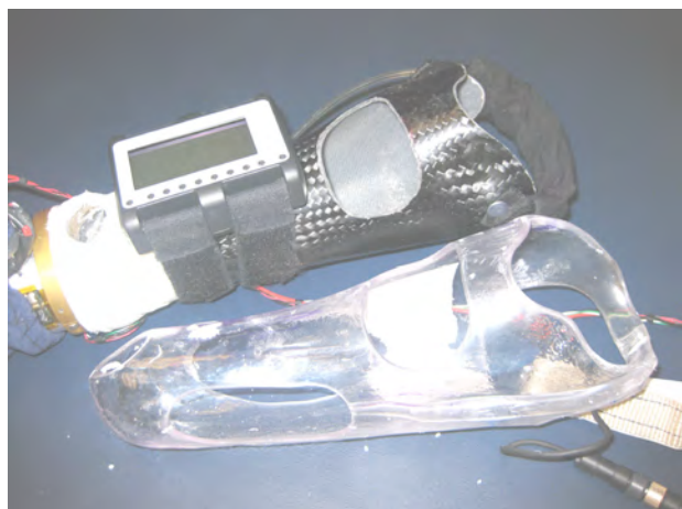
Figure 3: The completed arm with DEKA hand, and user display mounted on the forearm.
