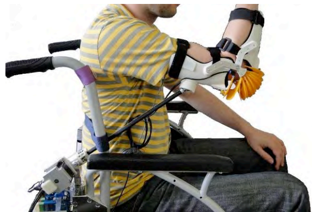
Figure 7: Test of the shoulder- and elbow modules
