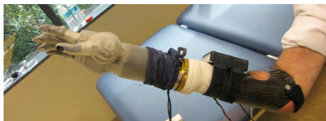
Figure 3: The completed arm with DEKA hand, and user display mounted on the forearm.
