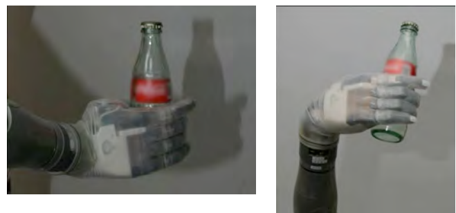
Figure 4. Examples of the hand in wrist extension-radial deviation position to place a bottle on a surface below the passive elbow position (left) and in a flexed, ulnar deviation position to place a bottle on an overhead shelf (right).
