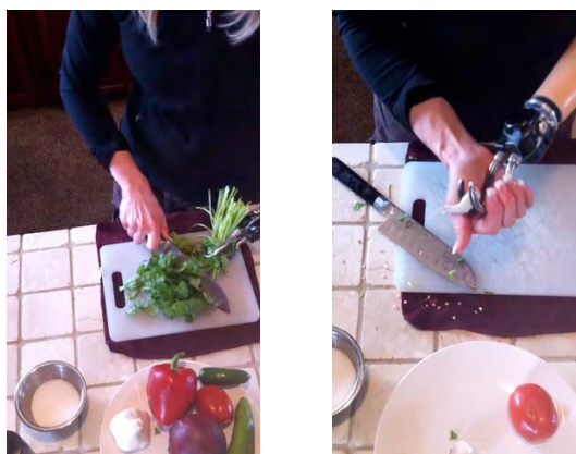
Figure 4&5 - Cooking tasks demonstrate the water-resistance of the ETD as well as the strength of the Titanium hook fingers.
