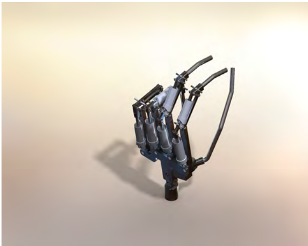
Figure 1: The CAD-design of the hydraulic hand
