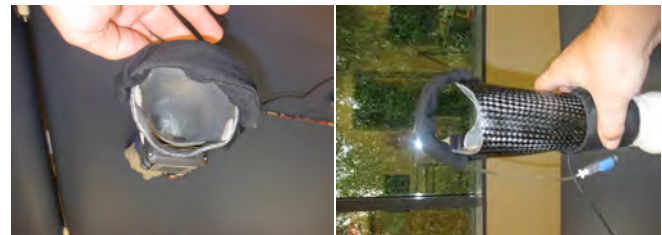
Figure 1: Proximal and Posterior view Socket with Dynamic Load Strap. The posterior strut was comprised of the dynamic load strap. The attachment nozzle for the airbladder is shown in the lower right.
