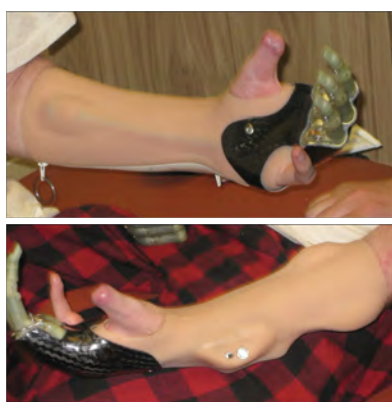
Figure 2: Partial hand prosthesis with ProDigits.
