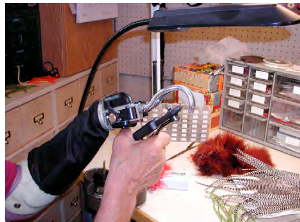
Figure 2 - Flexion and extension allow the ETD to function as a positional vice, e.g., for fly-tying.
