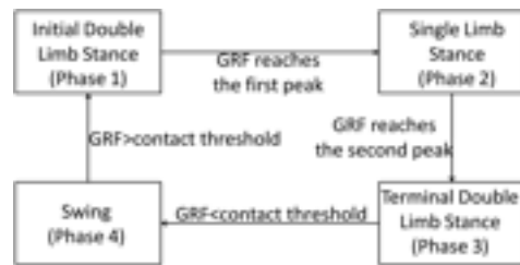
Fig. 3. The real-time gait phase detection criteria
