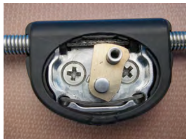
Figure 2: Mechanical Sure-Lok cable lock with top removed
