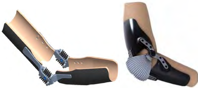
Figure 4: Design study of the OrthoJacket powered orthosis with two FFAs on each side of the elbow joint to enable both powered flexion and extension of the elbow (le.) and design with one FFA under use of pressure and vacuum (re.)
