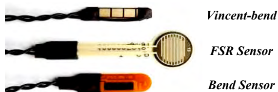
Figure 2: Sensors: Vincent-bend , FSR Sensor (Touch-Pad) and Bend Sensor in compare
