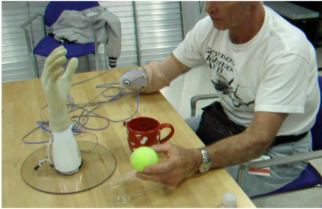
Figure 2: Remote control of prosthesis using pattern recognition
