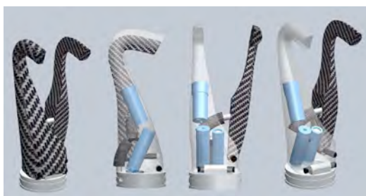
Figure 4: Mock up of a child sized prosthesis (approx. 100mm total length), including all hydraulic components.
