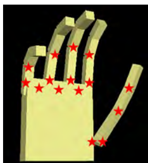
Figure 2: Virtual hand model with 15 articulating joints
