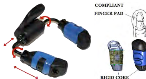
Figure 2: Epicondyle Contact Configuration
