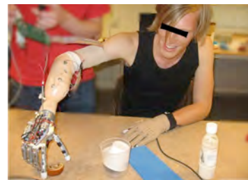
Fig. 1 Amputee reaching an object wearing SmartHand. The unnatural reaching posture of the arm caused by the lack of the 3 degrees of freedom of the wrist/forearm is clear from this picture.
