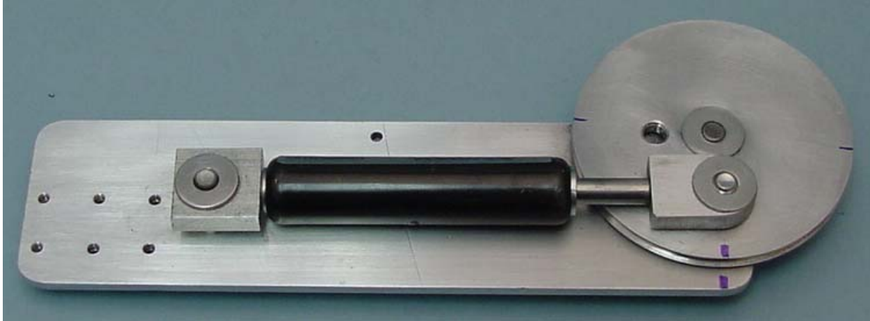
Figure 6. The gas strut is shown in the position of maximum tangential force. The cable from the bearing parallels the long axis of the assembly. The two marks show the location of the maximum force position of the pulley. Note that two thinner marks for zero compensation are on a line about 15^\circ from line between the pulley and strut axes.
