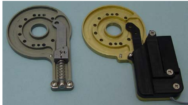
Figure 6. The base plate supplied with the manual joint on the left is held in place by only two screws making it easy to substitute the electric unlock base on the right.
