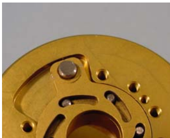
Figure 2. Unlock cam ring drives six plungers. The large pin is driven by the puller.
