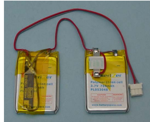
Figure 3. Safety features of a typical battery. The cell on the left mounts the safety circuit that monitors each cell separately. A Polyfuse on the right limits short circuit current and prevents over heating.
