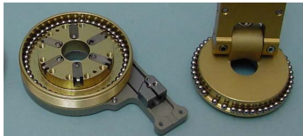
Figure 3. Six plungers move outward to engage slots between 36 posts in rotor. The large diameter ball races withstand the full 50 ft-lb (68Nm) design torque.
