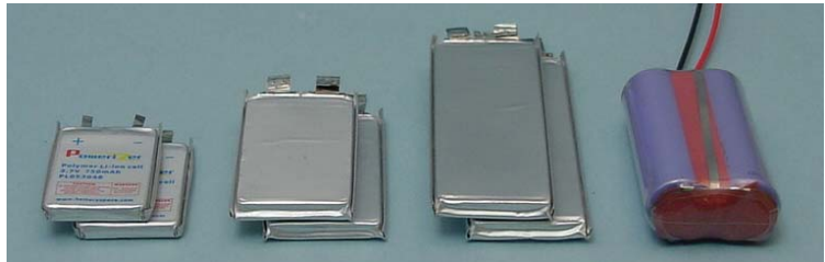
Figure 2. A pair of 750 mAh cells (30 mm wide, 44 g) compared with larger pairs 1350 mAh (33 mm, 66 g) and 2100 mAh (36mm, 88 g) and a 2000 mAh cylindrical pack (Two 18 mm cells, 98g).
