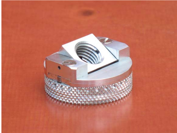
Figure 1. The new WILMER 2-DOF-wrist prosthesis for toddlers. It provides passive wrist flexion and passive wrist rotation.
