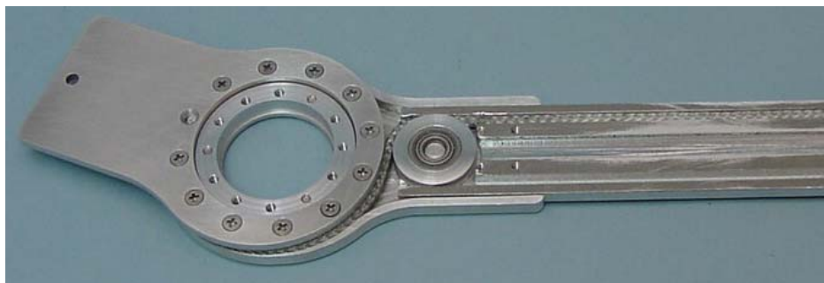
Figure 3. The flexion bearing showing a cable in the pulley groove of the large-diameter outer race. An idler pulley redirects the cable to pass down the thin strut on the right into the arm. This strut attaches to the compensator below the remaining limb.
