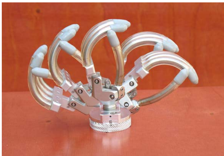
Figure 2. The new wrist provides 120^\circ flexion-extension in 30^\circ intervals.
