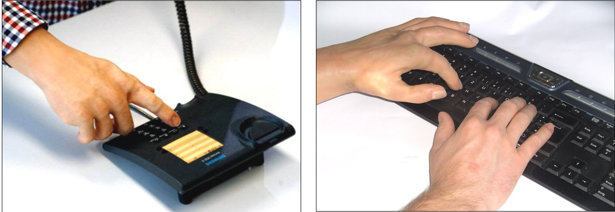
Fig. 1a and 1b: Options to operate a keyboard with the new prosthesis. Either the index is extended and the other fingers flexed, or vice versa.
