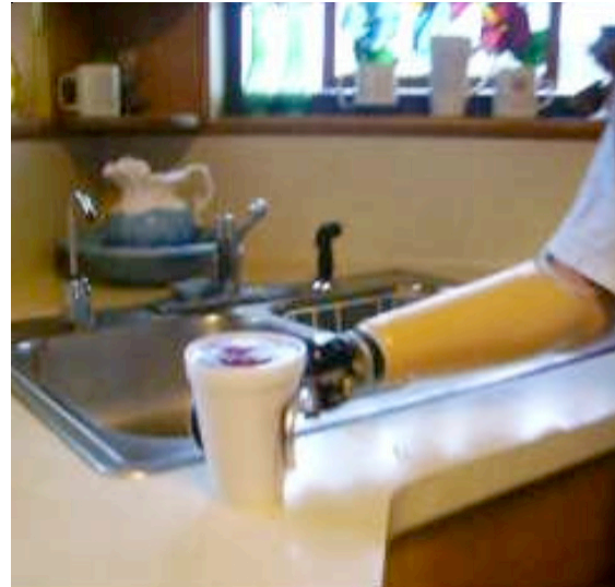
Figure 4 - Actual installation of the feedback element, producing vibration sensed by the wearer's skin, is a process of trial and error, at times. Several locations were used, some only temporarily, in the check socket stage of fitting with this wearer, including the location shown at left. The finished prosthesis, shown at right then could accommodate the vibration device at the preferred location, although changes are still possible if accommodation is experienced by the wearer, resulting in diminished sensation by the wearer. This prosthesis includes the GFF with an Electric Terminal Device (ETD), which also has the advantage of not requiring a glove or hand shell.
