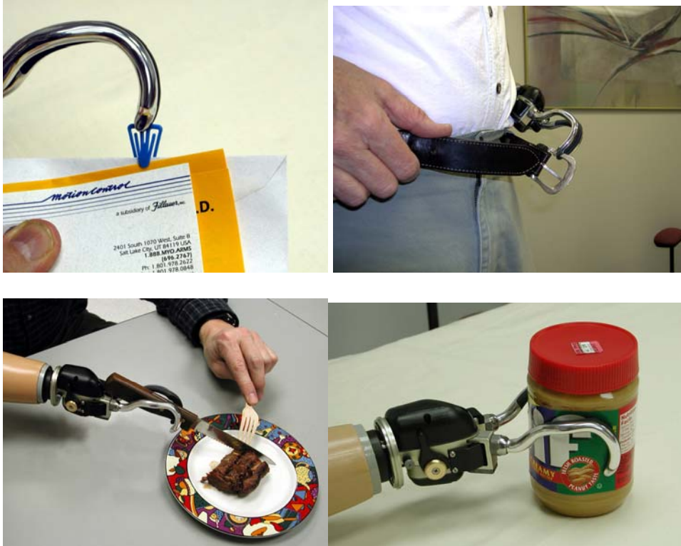
Fig. 5 Some of the advantages mentioned by ETD wearers were the fine tips, visibility of the curved shapes, high gripping pressure possible with the narrow finger shapes, and wide opening.
