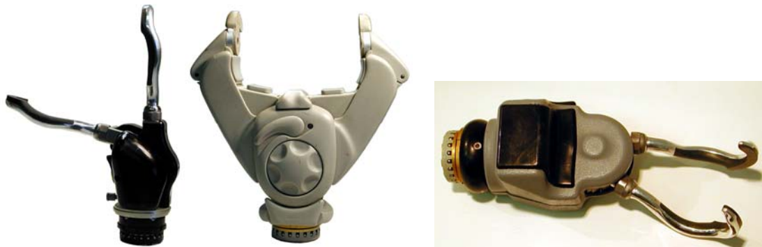
Fig. 6. The ETD compared to the Otto Bock Greifer and Hosmer Synergetic Prehensor.
