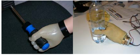
Fig. 1: The silicone prototype and the polyurethane prototype performing a grasp
