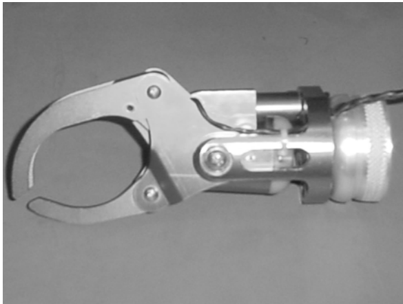
Figure 2 - The mechanical hand with the leadscrew decelerator
