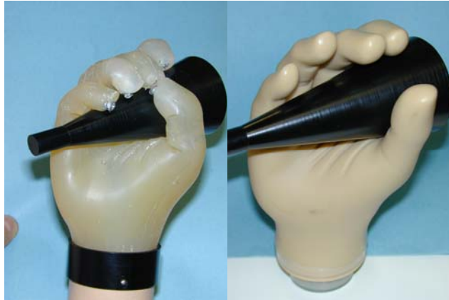
Fig. 6: The enveloping grasping of the Soft and compared with the grasp of a commercial prosthesis with rigid transmission
