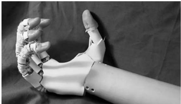
Fig. 1: The first prototype with 14 dependant DOF's.
