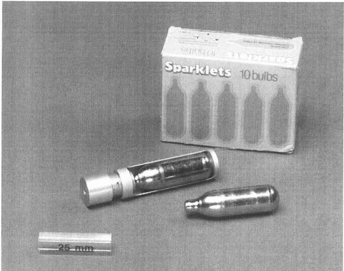
Figure 2: The bi-phasic hand prosthesis is powered by compressed CO 2 obtained from disposable cartridges. The desired supply pressure level is attained through a pressure-reducing valve, shown here at the left in the figure.
