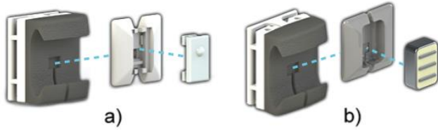
Figure 2: Exploded view of a) FSR and b) surface EMG electrode into panel system via removable inserts.
