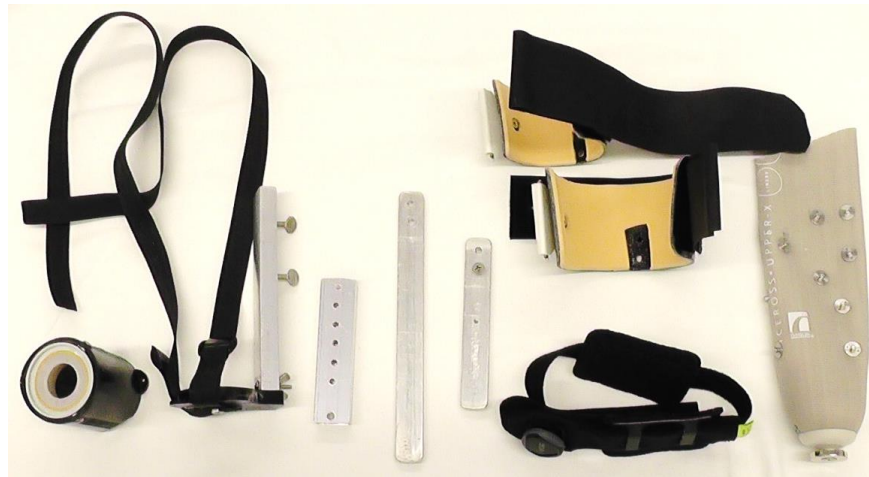
Figure 4: Photograph of all components of the second iteration of the universal transradial fitting frame broken down to show each part individually.
