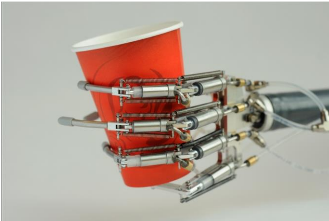
Figure 1 - The prototype of the Delft Cylinder Hand. It has four adaptive fingers actuated with two hydraulic cylinders in each finger, except for the little finger which has only one hydraulic actuator. The springs return the fingers to the open position at rest, and partly compensate for the counteracting forces of the cosmetic glove (not shown in the picture) as well. The cylinders in the hand receive the pressurized hydraulic fluid from a master cylinder incorporated in a shoulder harness.
