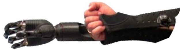
Figure 5: A photograph of the able-bodied simulator.
