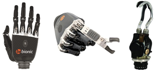
Figure 4: The 3 terminal devices used for testing: standard Bebionic hand (left), Bebionic with Pointdexter (center), and ETD (right).
