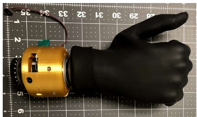
Figure 1: Prototype VAPI with iLimb Hand
