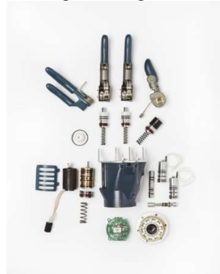
Figure 2: MyHand Advanced Hydraulic Design
