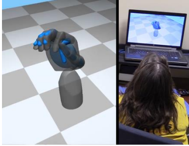
Figure 2: P2 performing the dextrous 2 DOF target matching task by simultaneously and precisely matching the positions of the virtual index and MRS fingers ( grey ) which she had position control over to their cued positions ( blue ). The cue turned green to indicate successful positioning of the fingers.
