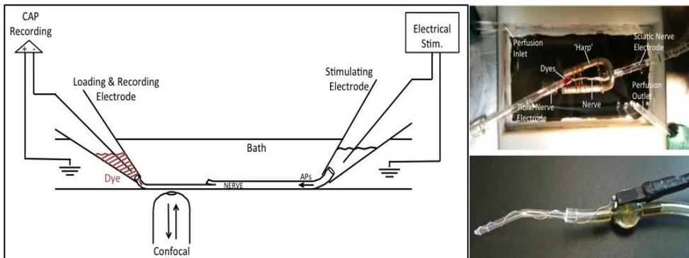
**Figure 4:** Nerve dye-loading, electrophysiology & imaging configuration
