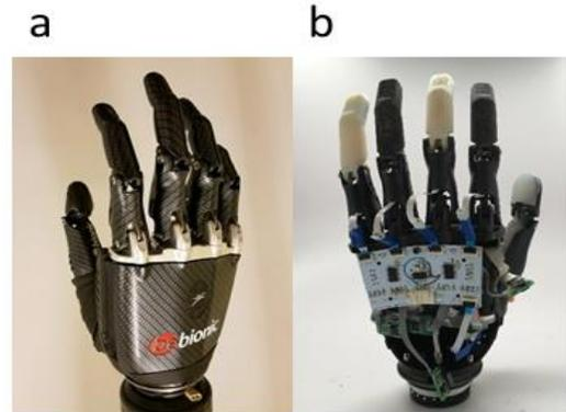
**Figure 5:** (a) Commercially available Bebionic v2 hand (b) Modified Bebionic hand used for finger actuation experiments. Custom electronics were installed in order to control individual motors within the prosthesis. The Bebionic has motor encoders that can measure finger position and be used in closed-loop control.
