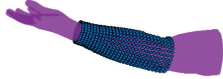
Figure 2: Sensors arrangement around the forearm, extracted from the CAD model. A grid of  $N = 840$  sensors was used to collect the magnetic field generated by the implanted magnets. The longitudinal and radial step of the grid was set to 10 mm and  $12^\circ$ , respectively.
