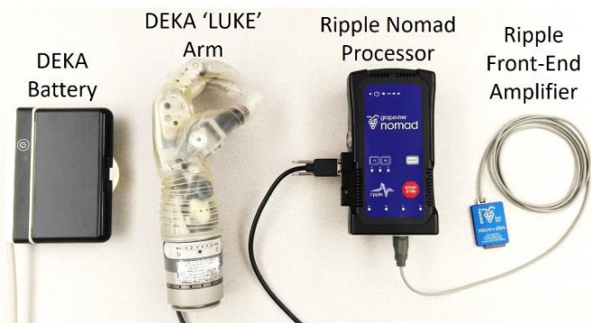
Figure 1 – Portable take-home system includes the DEKA LUKE Arm and battery, the Ripple Nomad neural interface processor and battery (hidden) and a front-end amplifier (amplifier for surface EMG shown here).
