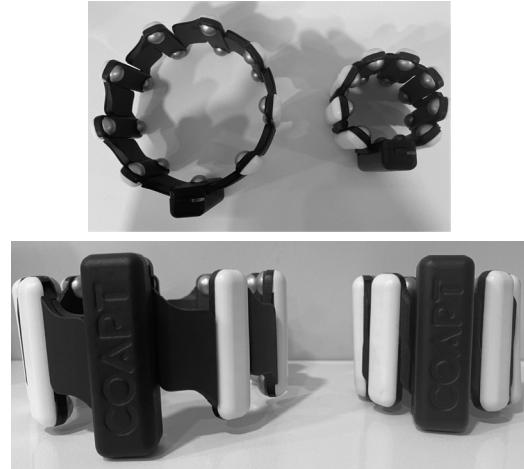
Fig. 1: A standard and larger sized EMG-embedded arm/leg cuff embedded with bi-polar electrode sensors for convenient acquisition of up to 8 muscle activity signals.
