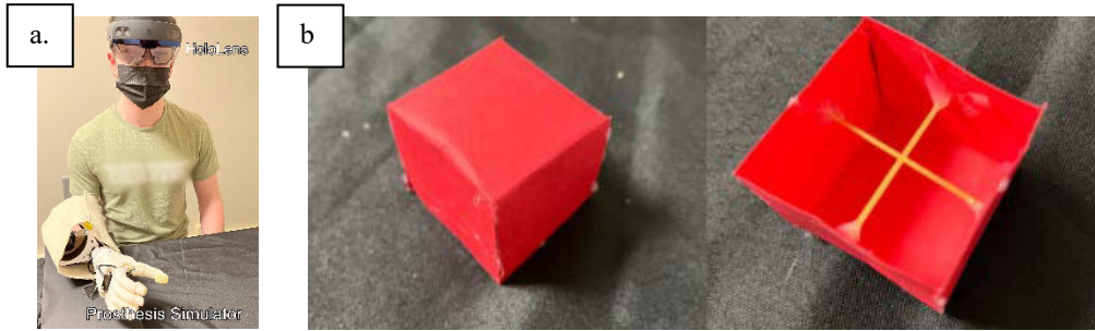
Figure 2: Experimental setup. A. Participants wore the HoloLens 2 while controlling a prosthesis simulator. b. Mechanical egg in grasp-and-hold task. Left , participant view. Right , underside showing intact pasta fuses [15].
