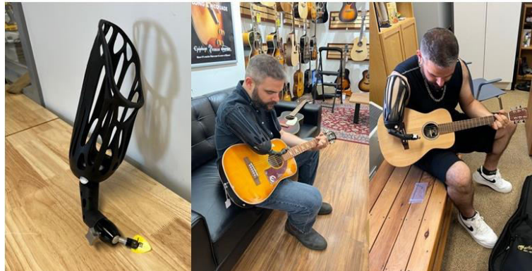
Figure 1: custom transhumeral guitar device
