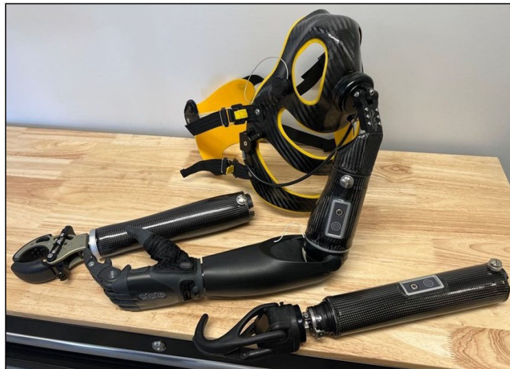
Figure 3: Final Prosthesis with three interchangeable arm segments
