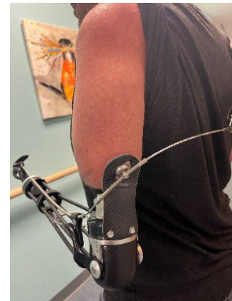
Figure 2: A rigid distal outriggers is used to mount the baseplate and retainer of a body powered prosthesis.
