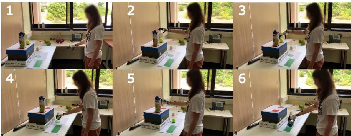
Figure 3: Time representation of a patient using the Hannes prosthesis during ADLs. Preparation of the wrist configuration to grasp an object (1), reaching the spherical object (2), adjusting the wrist FE to comfortably grasp the object (3), extend the wrist to place the object on the table (4), adjust the wrist PS to grasp a vertical object (5), adjust the wrist PS to place the object horizontally on the table (6).
