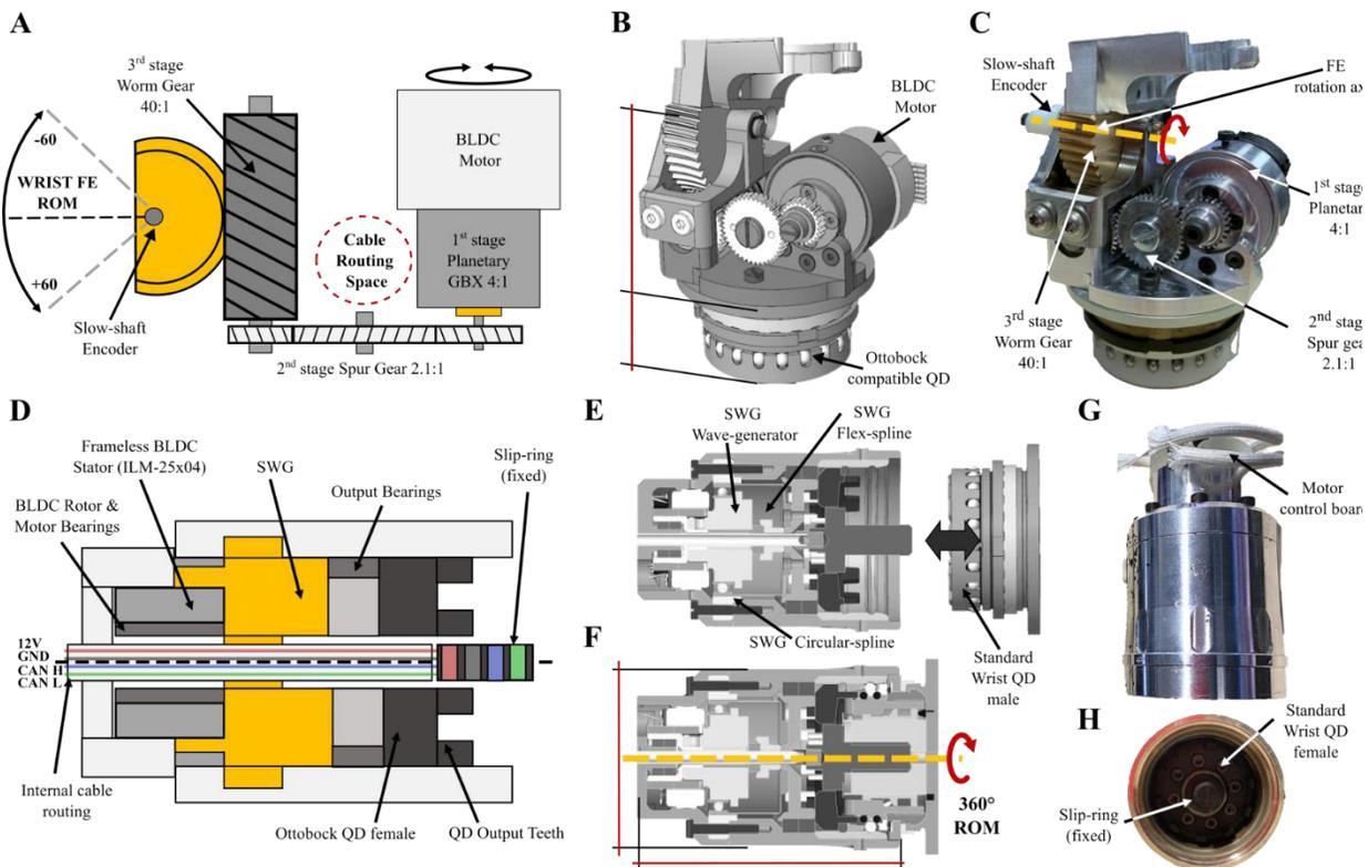
Figure 1: Wrist FE: **A)** Schematical representation of the adopted mechanism; **B)** Computer-aided design of the wrist device; **C)** Actual representation of the wrist device. Wrist PS: **D)** Schematical representation of the adopted mechanism; **E-F)** Computer-aided design of the wrist device; **G-H)** Actual representation of the wrist device.
