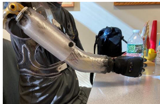
Figure 2: Novel shoulder disarticulation style prosthesis in its shortest position to function while seated at a table
