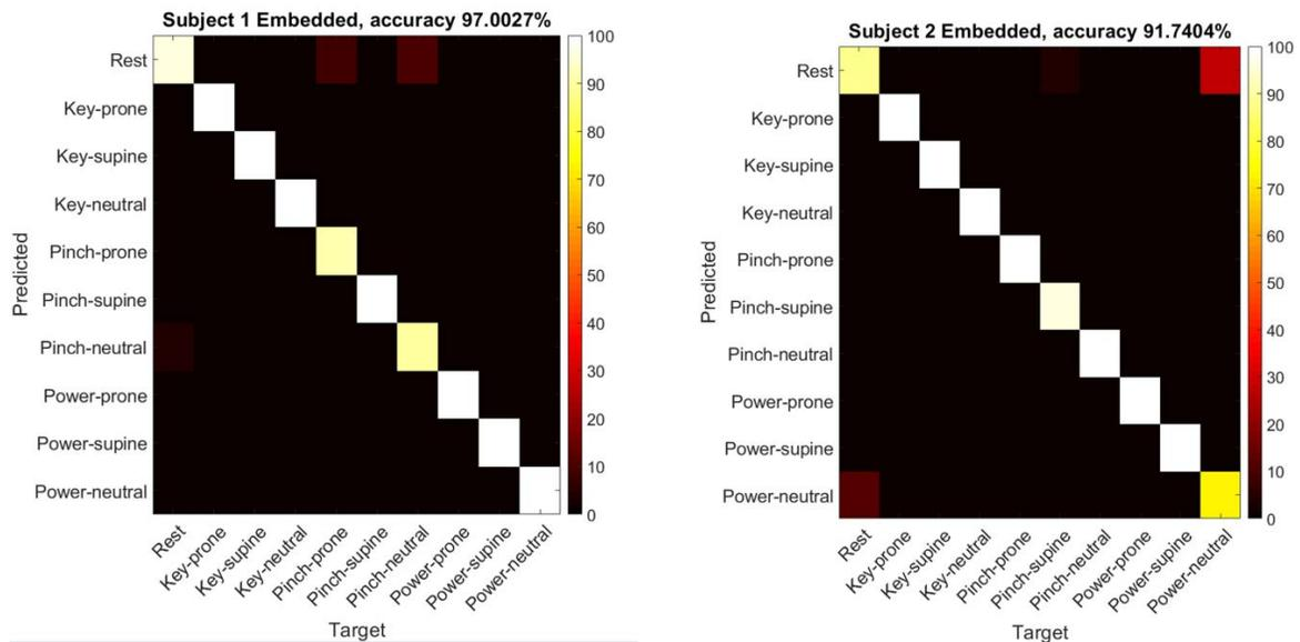
Figure 3. Offline grasp classification accuracy obtained using an embedded processor when testing two able-bodied subjects.
