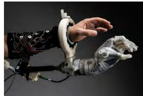
Figure 2: Prosthesis Setup. Participants wore an sEMG sleeve around their forearm and held a prosthesis via bypass socket fit around their wrist.
