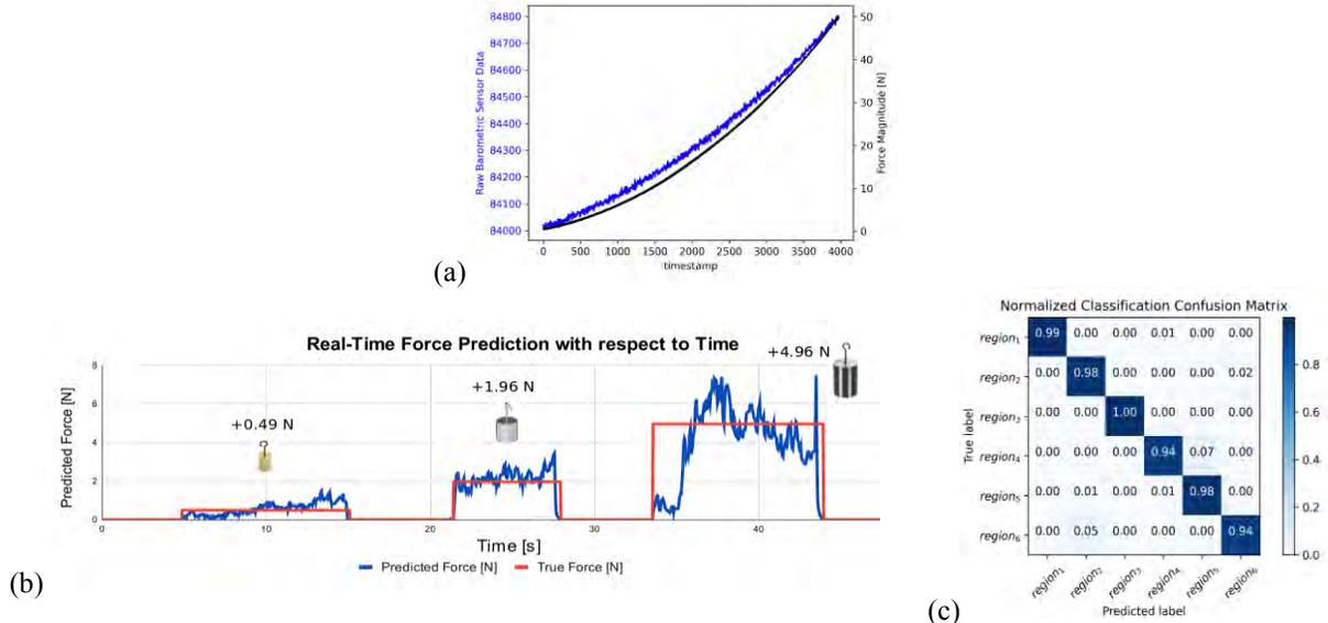
Figure 4: (a) Raw barometric signal after applied load. (b) Real-time onboard force prediction results using three dead weights. (c) Confusion matrix representing offline classification performance.
