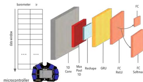
Figure 3: Neural network model; the architecture is interpreted from left to right.
