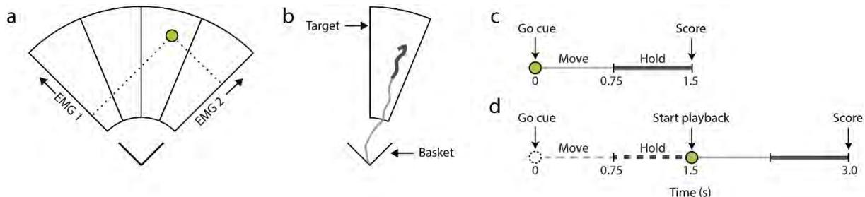
Figure 1: The MCI task. (a) The 2D myoelectric interface space. Cursor position shown in green. (b) A representative cursor trajectory from basket to target. Thick cursor mark denotes the hold period. (c-d) Task timing structure for the Concurrent and Delayed conditions, respectively, denoting cues and the move, hold and playback periods. Dashed traces correspond to the ‘blind’ control input window. Solid traces indicate when the cursor’s motion was visible during a trial.
