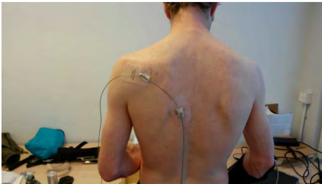
Figure 4 – The skin anchors placed on the body of a test subject. The cables are connected to the experimental set-up used to verify the idea behind the haptic interface.
