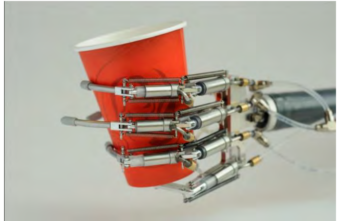
Figure 2 - The prototype of the Delft Cylinder Hand. It has four adaptive fingers actuated with two hydraulic cylinders in each finger, except for the little finger which has only one hydraulic actuator. The springs return the fingers to the open position at rest, and partly compensate for the counteracting forces of the cosmetic glove (not shown in the picture) as well. The cylinders in the hand receive the pressurized hydraulic fluid from a master cylinder incorporated in a shoulder harness.
