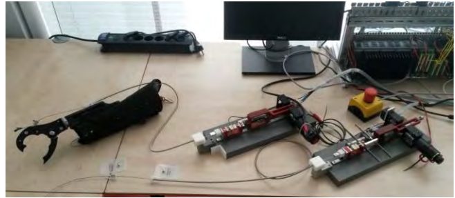
Figure 5 – The experimental set-up. On the left the prosthetic simulator; in the middle and right part of the figure the master-slave unit is shown. Also visible are the cables and on the foreground, the skin anchors.
