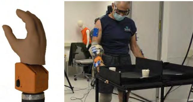
Figure 1: a) Device used for the study. b) Participant wearing the device, in “home” position, ready to begin the Cup Transfer Task.
