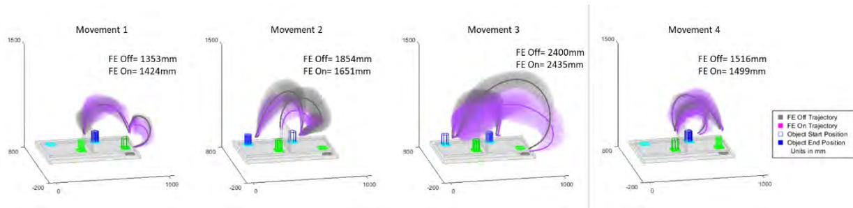
Figure 3: Trajectory of the prosthetic hand during the 4 movements: average with  $\pm 1$  standard deviation (SD) shaded. The mean overall distance of each curve (in mm) is shown for both conditions.
