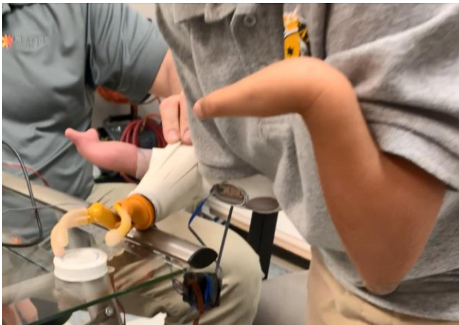
Figure 3: Dynamic assessment of the internally rotated prosthetic forearm to ensure optimal upper limb function.
