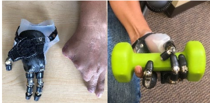
Figure 5: (Left) Patient's presentation and prosthesis with Point Thumb, two Point Digits, and one Point Partial. (Right) Patient lifting a weight with prosthesis.
