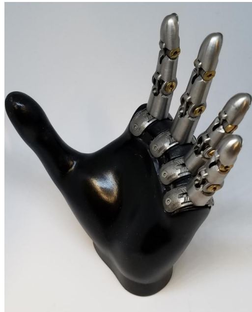
Figure 1: A depiction of the miniature digits spanning lengths of 55mm (little finger) to 75mm (middle finger) on a full hand model.
